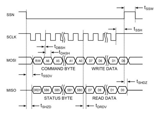
Figure 4-6: SPI Timing Diagram, CPOL = CPHA = 1
