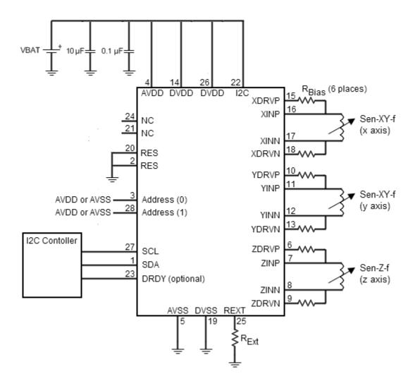
Figure 4-2: RM3100 reference schematic – l<sup>2</sup>C Configuration
