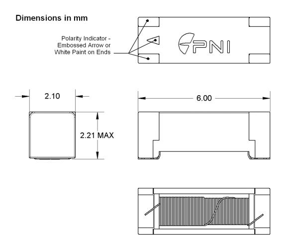
Figure 3-1: Sen-XY-f Sensor Dimensions
