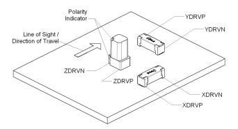
Figure 4-4: RM3100 North-East-Down (NED) Sensor Layout
