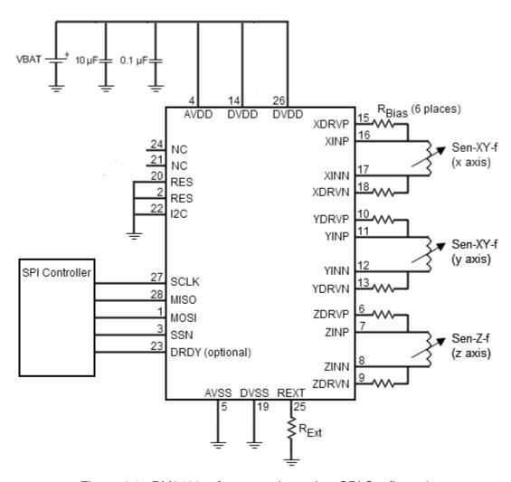
Figure 4-1: RM3100 reference schematic – SPI Configuration
