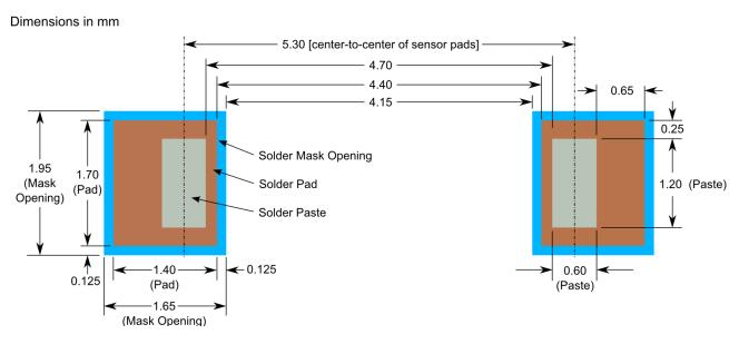
**Note:** PNI recommends a 5 mil stencil. The solder paste area is much smaller than the pad to reduce sensor tilt and misalignment. The above layout allows for rework: for minimal footprint, contact PNI.
