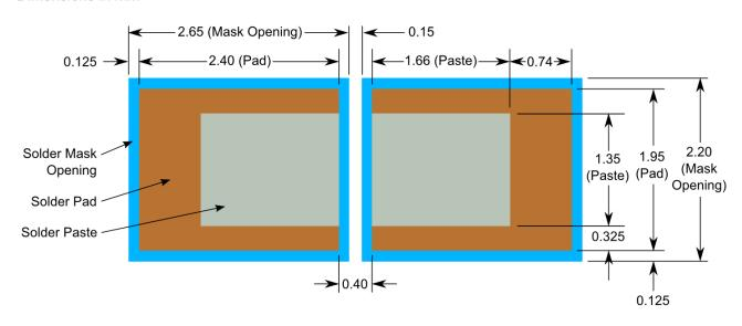
**Note:** PNI recommends a 5 mil stencil. The solder paste area is much smaller than the pad to reduce sensor tilt and misalignment. The above layout allows for rework: for minimal footprint, contact PNI.
