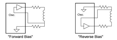
Figure 4-3: LR Oscillator Circuit Biasing Diagram
