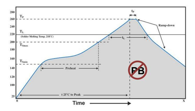
Figure 3-9: Recommended Solder Reflow Profile
